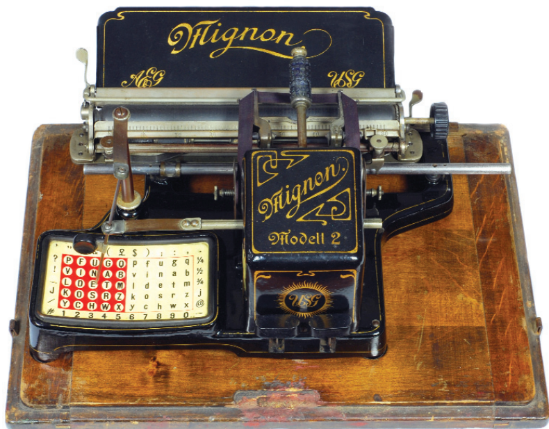
Mignon 2 - Berlin, Germany - 1905: Despite its unusual appearance, the Mignon typewriter embodied a very clever design, giving a smooth and fast operation. The index plate and the type-cylinder could be changed, allowing for different languages and fonts.
