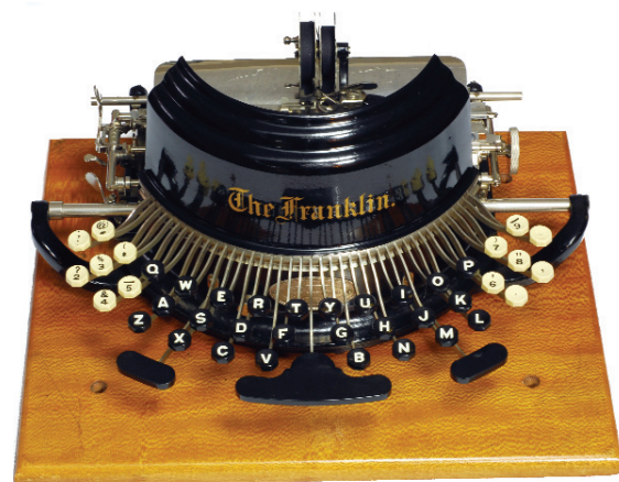
Franklin 2 - Boston - 1892: Like the Bar-Lock typewriter, the type-bars stand vertically behind the curved shield and swing down to strike the top of the platen.
